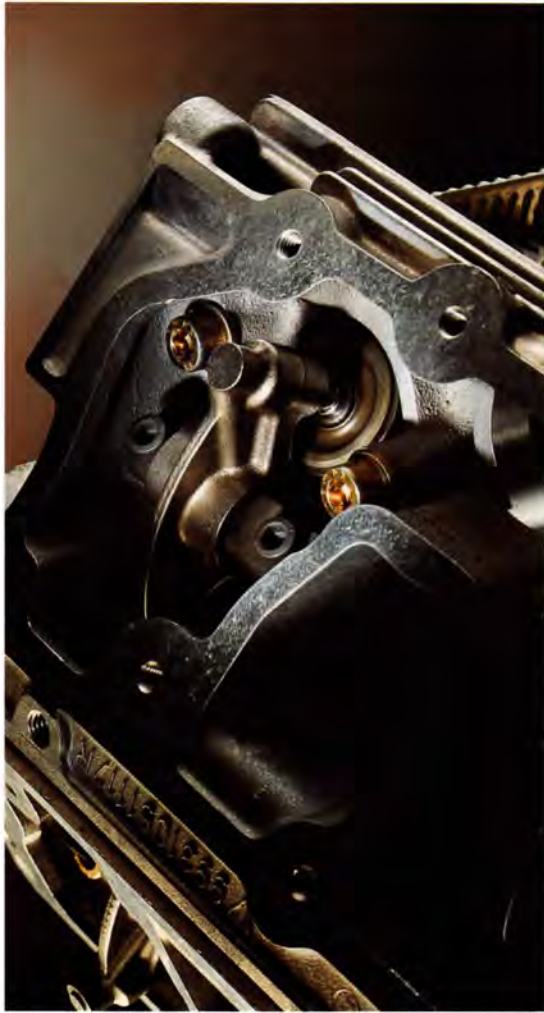
On the new 911 Turbo, valve play is balanced hydraulically to save the time and expense of regular valve adjustment intervals.
