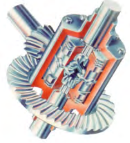
The mechanical limited slip differential lock reduces load factor shifts when cornering. The locking ratio for the rear axle is 25 %, increasing to 40 % when easing off on the accelerator.
