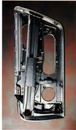
Since 1985, all Porsche models have featured reinforced side impact door sections. Premium VZA German steel is used in the new 911 Turbo for an added measure of safety.
